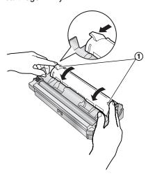
**10** Make sure that the triangles (①) match, to install the toner cartridge correctly.
